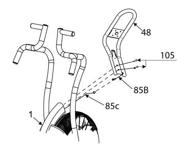
Step 6: Assembling the Cockpit and Bottle Holder
