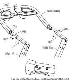
Inside view of the right side Handlebar Assembly mounting bracket fully seate Left side is a mirror image of the right side.
