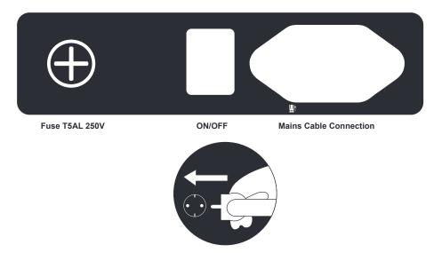
Connect the mains cable to the connection on the massage chair. Then connect the mains plug on the mains cable to a power socket.
